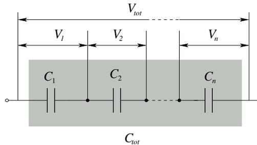
Figure 5.8: Capacitors in series.
