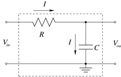
Figure 6.4: RC low-pass filter circuit.
