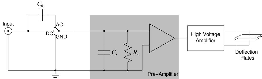
Figure B.3: Oscilloscope input impedance representation using ideal components (gray box). Input channel coupling is also shown.
