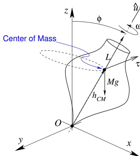
Figure 2.3: Precession of the top. In this sketch  $\vec{\tau}$  is parallel to the  $y$  axis and is pointing to the negative direction of the  $y$  axis. The vector  $\vec{h}_{CM}$  is in the plane  $Oxz$
