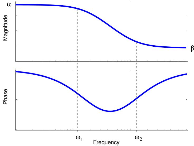
Figure B.5: Qualitative transfer function from the under compensated probe input to the oscilloscope input before the ideal amplification stage. As usual, the oscilloscope input is described having an impedance  $R_s || C_s$ .
