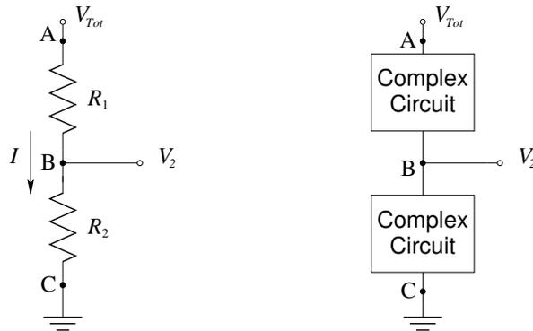
Figure 5.12: Simplest and complex voltage divider circuit.
