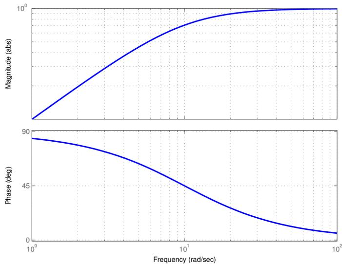
Figure 6.7: CR high pass filter circuit transfer function.
