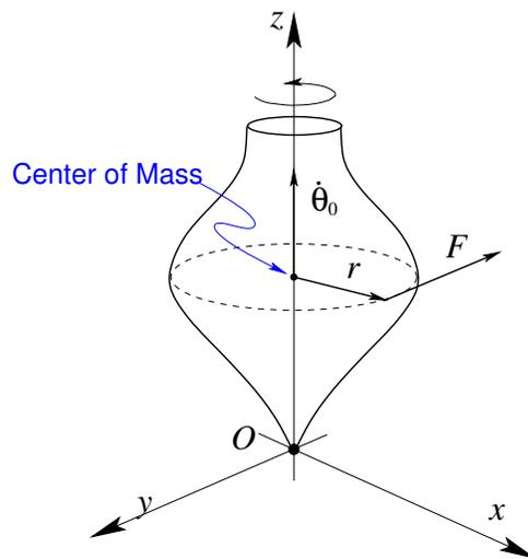
Figure 2.1: Top subject to an external force  $\vec{F}$  which produces a torque  $\vec{\tau} = rF\hat{z}$ .
