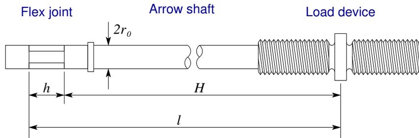
The load device is designed to place the load symmetrically respect the point A keeping the length of the leg  $l$  constant.
