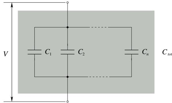
Figure 5.7: Capacitors in parallel.
