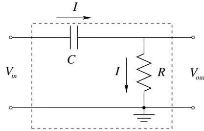
Figure 6.6: CR high pass filter circuit
