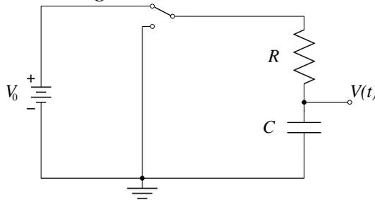
2. Choose the values of  $R$  and  $C$ , with  $R \ll 1\text{M}\Omega$  to get the time constant to be  $\tau = 1\text{s}$ . Prove that  $\tau$  has the dimension of a time (hint: use eq.(5.2) and (5.1)).
