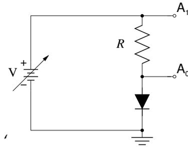
1. Determine the polarity and the turn on voltage of a germanium diode and a silicon diode .
