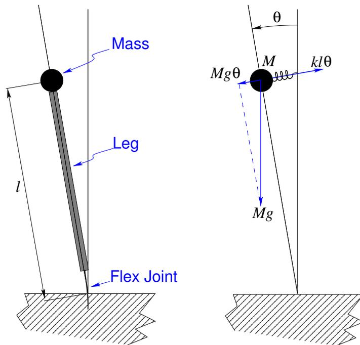
Figure 4.1: Simple model of the inverted pendulum.
