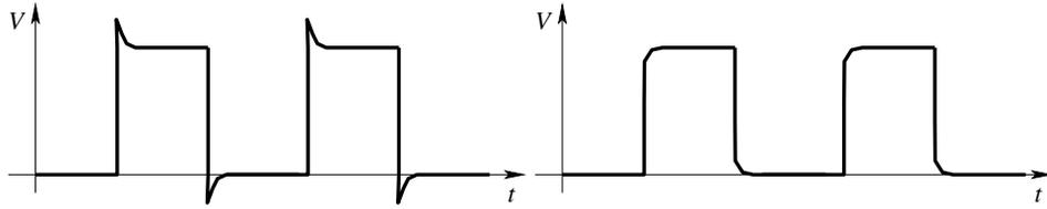
Figure B.6: Compensation of a passive probe using a square wave. Left figure shows an over compensated probe, where the low frequency content of the signal is attenuated. Right figure shows the under compensated case, where the high frequency content is attenuated.
