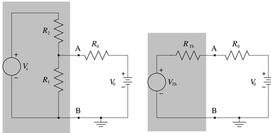
Figure 5.14: Thévenin equivalent circuit example
