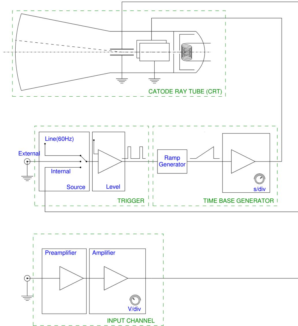
Figure B.1: Oscilloscope functional schematics
