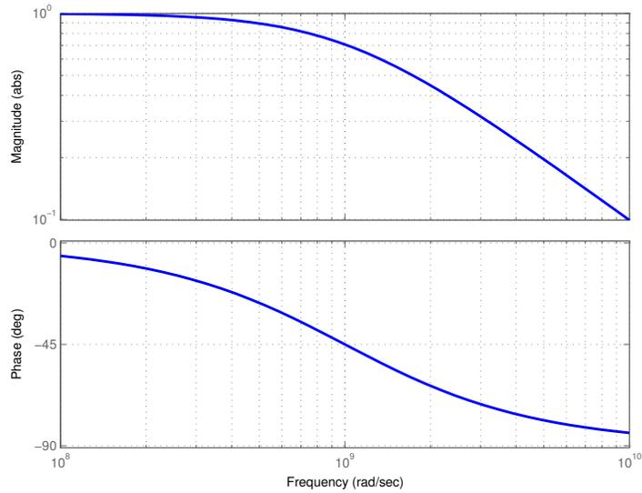
Figure 6.5: RC low-pass filter circuit transfer function.
