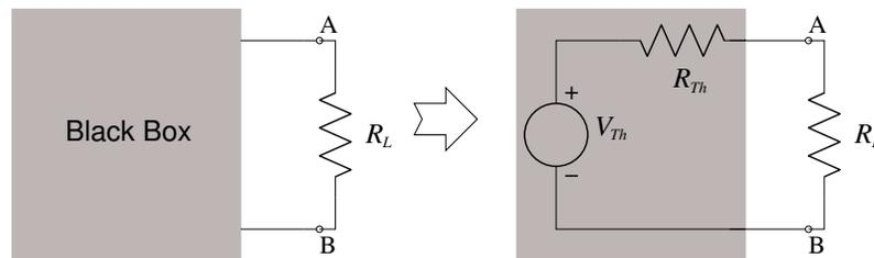
Figure 5.13: Thévenin equivalent circuit illustration.
