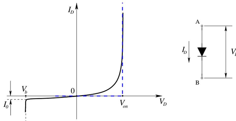
Figure 5.11: Diode characteristic (continuous curve), simplified diode characteristic (dashed curve), and diode standard symbol.
