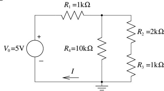
2. Find the equivalent Thévenin circuit for the following circuit respect to the point A and B :
