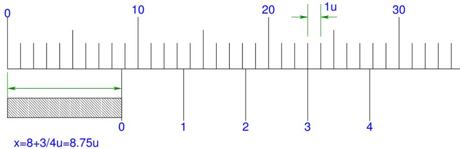
Figure A.2: Example of a vernier measurement with  $k = 5, n = 4 \Rightarrow \Delta x = 1/4$ units.
