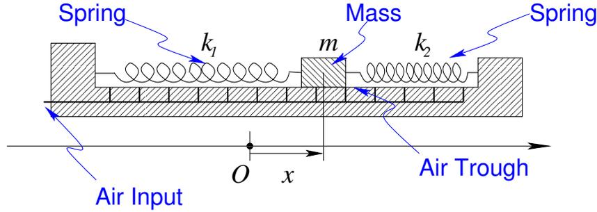
Figure 3.1: Mechanical oscillator sketch
