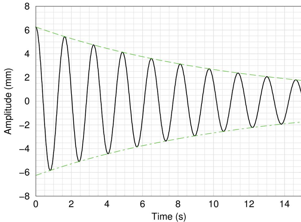
Figure 3.2: Mechanical oscillator ring down. The two exponentially decaying curves are the envelope of the ring down. The parameters used are typical of the real set-up,  $\omega_0 = 3.8 \text{ rad/s}$ ,  $\gamma = .17 \text{ s}^{-1}$ ,  $x_0 = 6.3 \text{ mm}$ .
