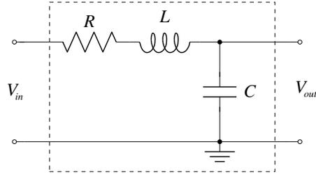
Figure 6.8: LCR series resonant circuit.
