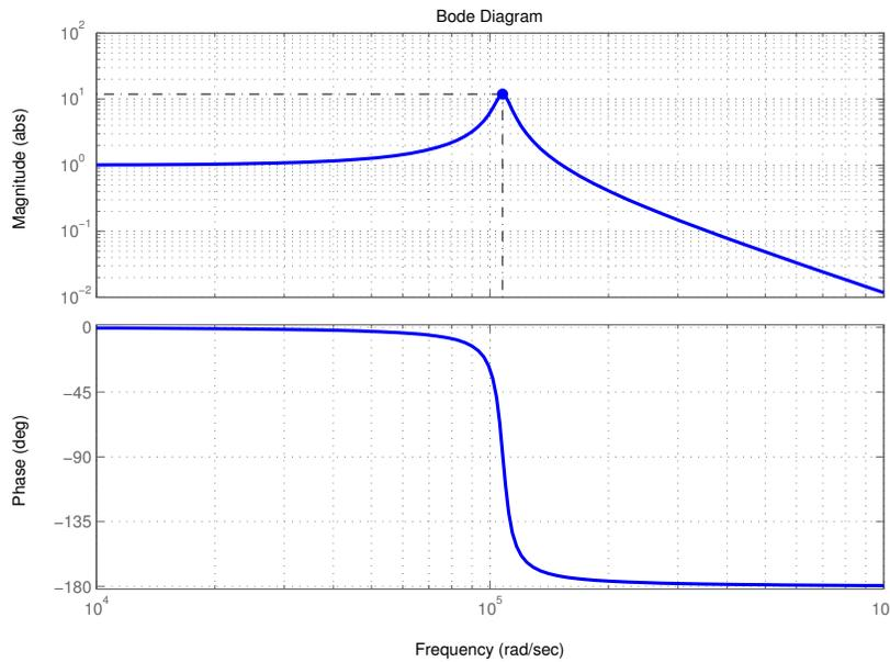
Figure 6.9: Transfer Function  $H_C(\omega)$  of the LCR series resonant circuit .
