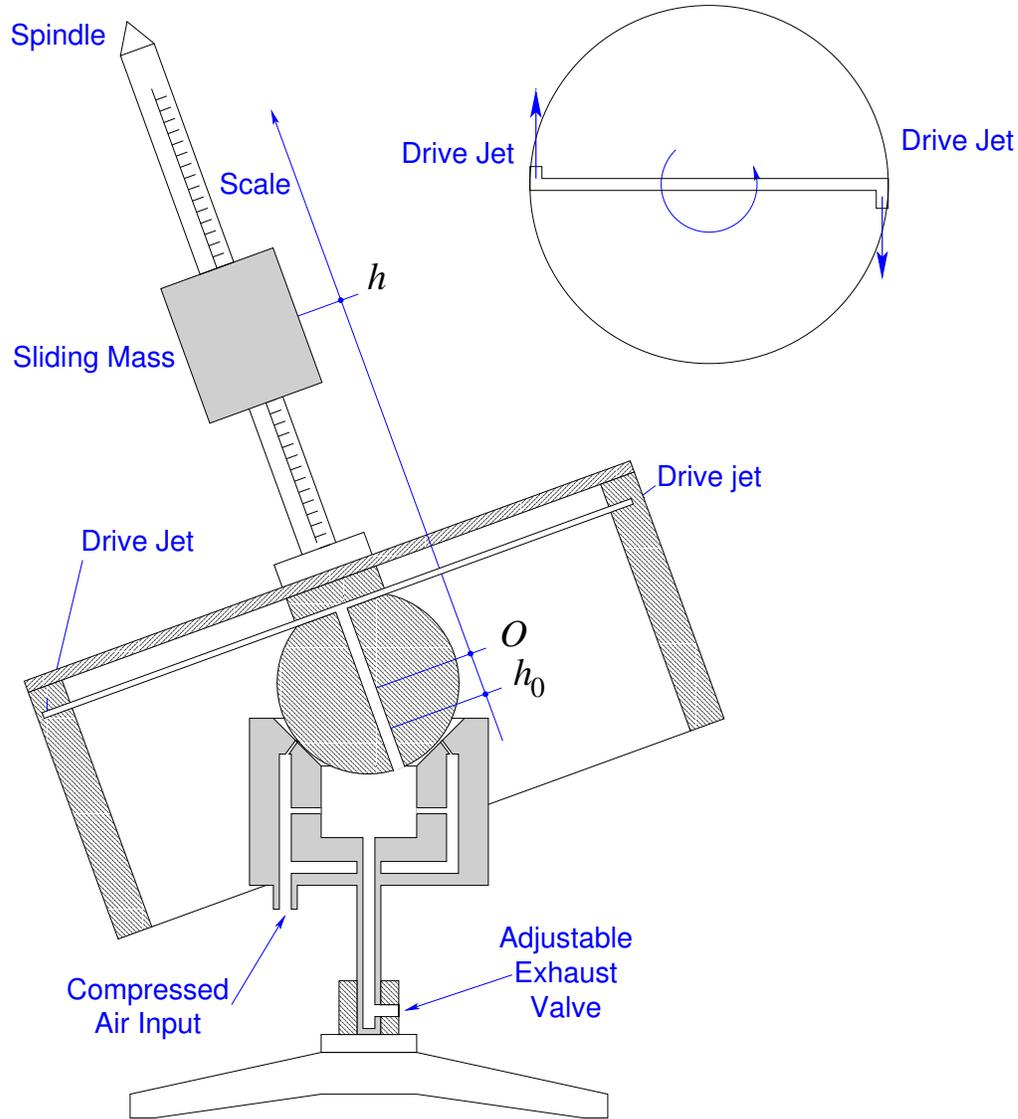
Figure 2.5: Maxwell Top schematic vertical cross section and top view cross section.  $O$  is the top's pivoting point and the sketched axis is oriented as indicated by the arrow. This implies that  $h_0$  is negative and  $h$  is positive.
