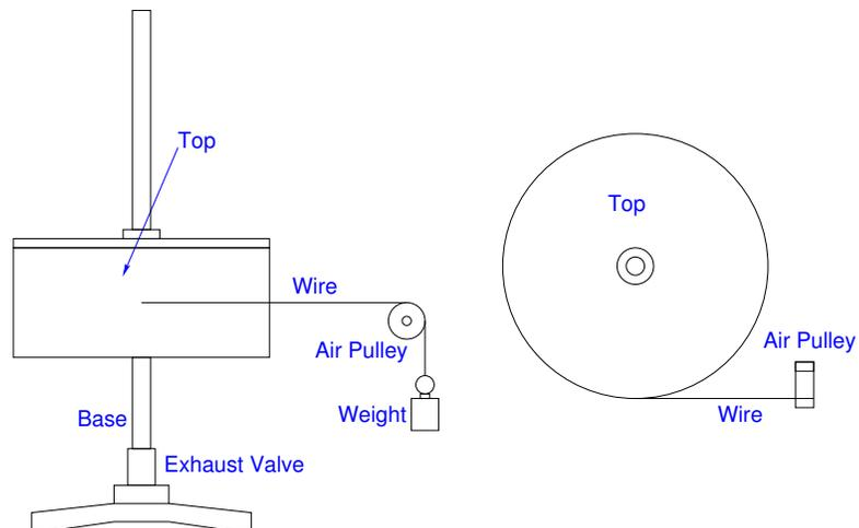
Adjust the exhaust valve to change the air-jets flow until the top reaches a state closest as possible to the equilibrium. Remove the
