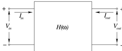
Figure 6.3: Two-port network circuit representation. The Voltage difference signs and current directions are conventional.
