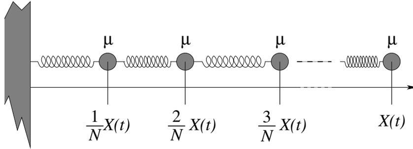
Figure 3.6: Simple discrete model of a spring.
