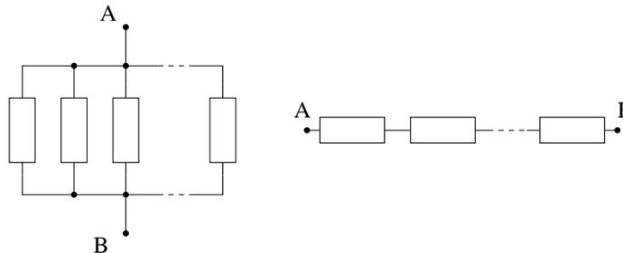
Figure 5.2: Considering the points A, and B, the components of the left circuit are in parallel, and those ones in the right circuit are in series.
