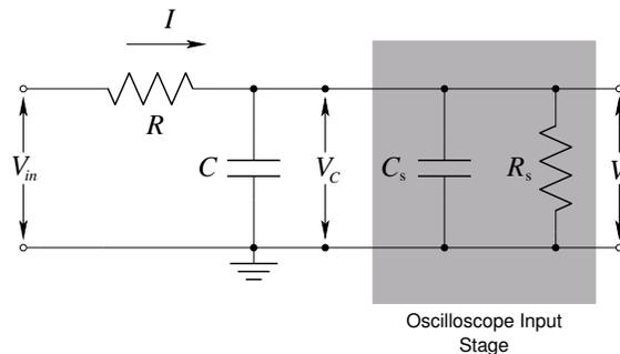
Find the voltage  $V_s(\omega)$ , and the angular cut-off frequency  $\omega_0$  of the transfer function  $V_s/V_{in}$  ( i.e. the value of  $\omega$  for which  $|V_s/V_{in}| = 1/\sqrt{2}$ ).
