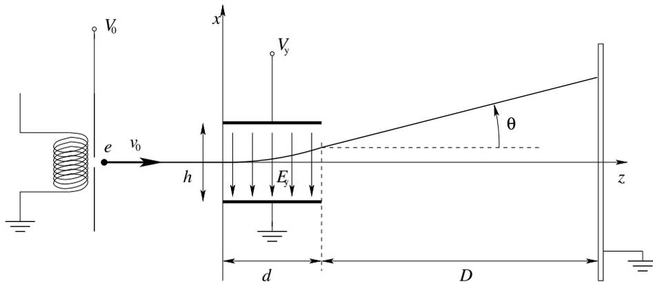
Figure B.7: CRT tube schematics. The electron enters into the electric field and makes a parabolic trajectory. After passing the electric field region it will have a vertical offset and deflection angle  $\theta$ .
