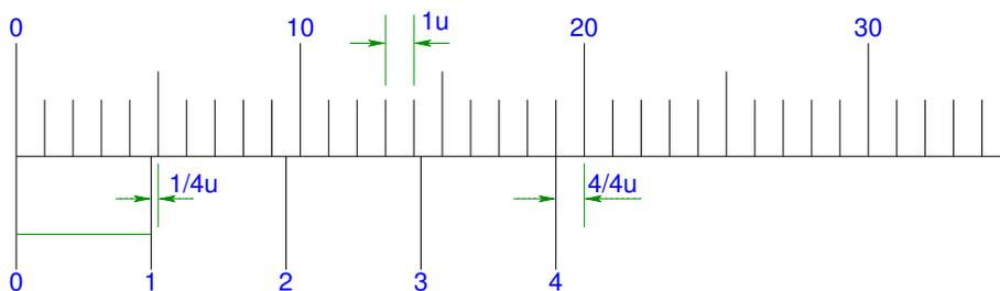
Figure A.1: Example of a vernier with  $k = 5$ ,  $n = 4$ , and  $\delta x = 1/4$  units. The two scales are aligned and the 4-th auxiliary division is aligned to the  $kn - 1 = 19$ -th division of the main scale.
