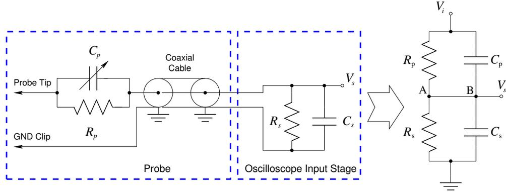
Figure B.4: Oscilloscope input stage and passive probe schematics. The equivalent circuit made of ideal components for the probe shielded cable is not shown.
