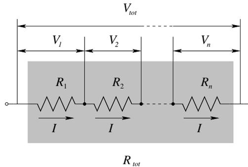
Figure 5.4: Resistor in series
