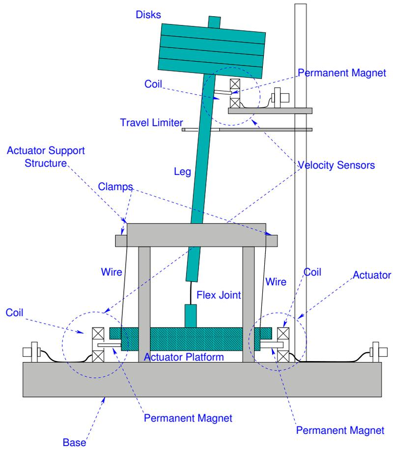
Figure 4.2: Inverted pendulum test bench .
