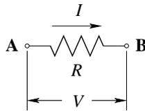
Figure 5.3: Resistor symbol
