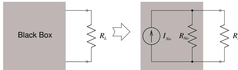
Figure 5.15: Norton equivalent circuit illustration.
