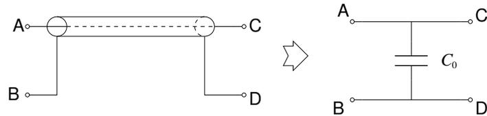
They have typical linear density capacitance  $\Delta C/\Delta l \sim 100\text{pF/m}$ . Single wires have usually smaller capacitance than BNC cables. Unfortunately, their capacitance strongly depends on how they are positioned one respect to the others.
