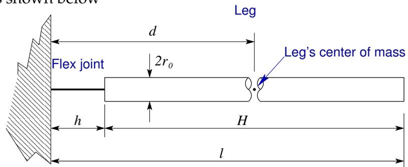
Compute the leg's moment of inertia  $I$  with  $m = 25\text{mg}$ ,  $l = 650\text{mm}$ ,  $h = 28\text{mm}$ , and  $r_0 = 5\text{mm}$ , and the systematic error on  $I$  if we neglect the leg's radius.
