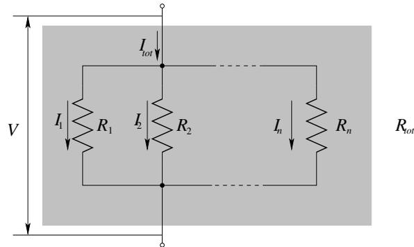
Figure 5.5: Resistors in parallel.
