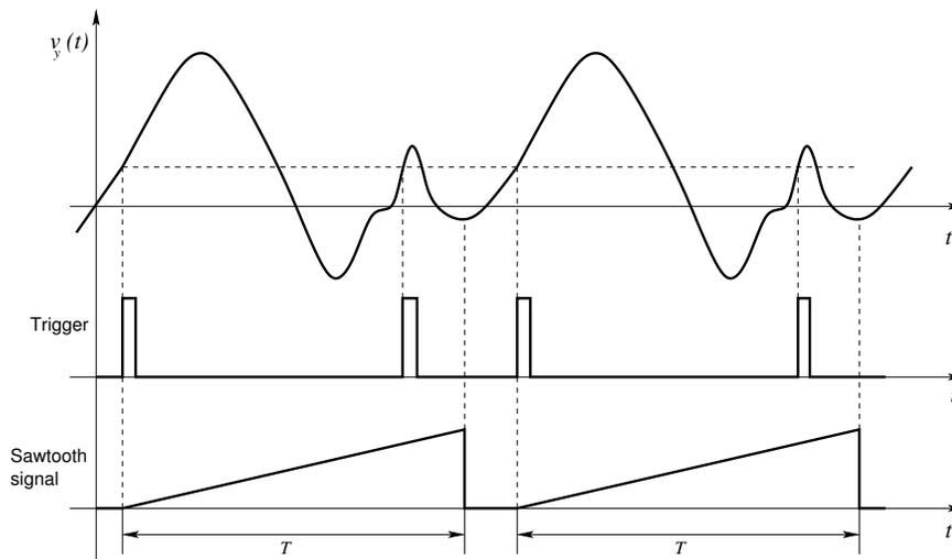
Figure B.2: Periodic Signal triggering.
