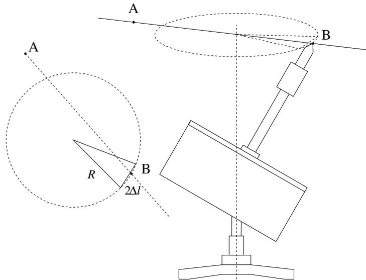
6. Using two points, **A** and **B**, to align the line of sight (see figure above), a careful student determines that the uncertainty of measuring where the spindle passes the pointer at **A** is  $\Delta l = \pm 2\text{mm}$ . If the radius of the precession orbit is  $R = 50\text{mm}$ , and the period is  $T = 60\text{s}$ , what uncertainty  $\sigma_T$  does this produce in the period  $T$ ? What fraction is  $\sigma_T$  of the total period  $T$ ?
