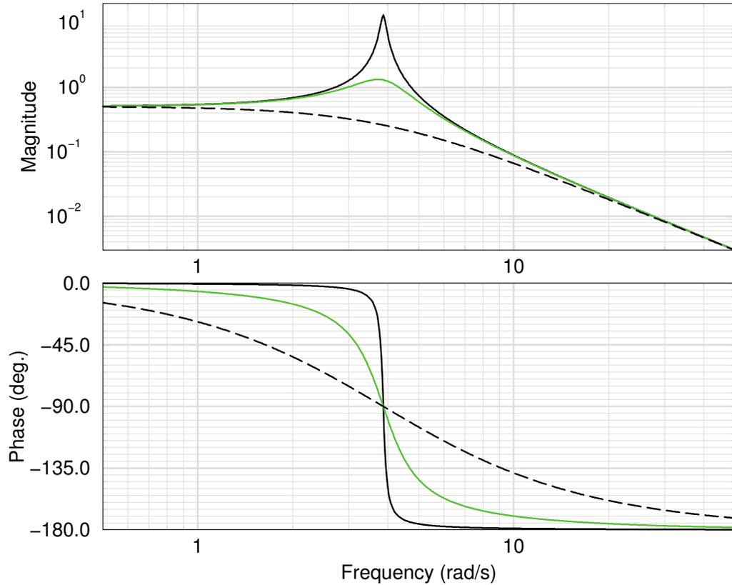
Figure 3.4: Amplitude and phase of the transfer function  $H(\omega)$  of the mechanical harmonic oscillator for three different values of  $\gamma$ .
