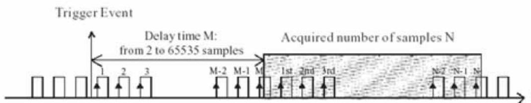
Figure 4.2: Delay-Triger Acquisition Mode
