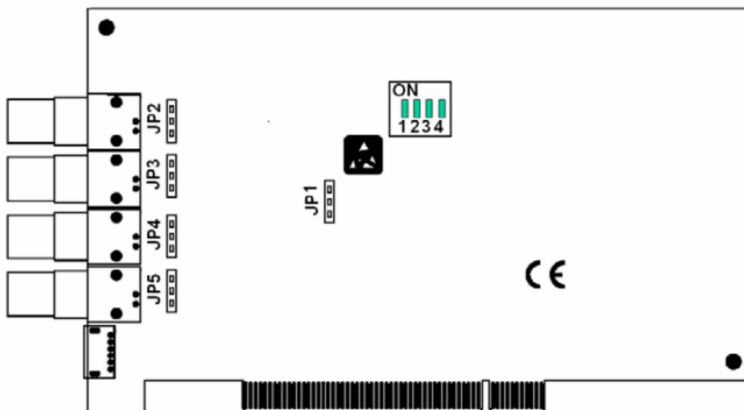
Figure 3.1: Card Connector, Jumper and Switch Locations
