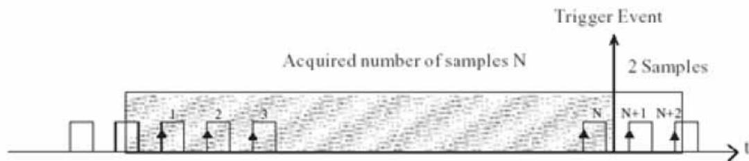
*Figure 4.4: Pre-Trigger Acquisition Mode*
